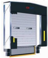
This type is designed to service a wide variety of trailer sizes and types, while providing full trailer access during the loading process. A gravity-biased, flexible frame yields to misguided trailers preventing costly building and shelter damage.
